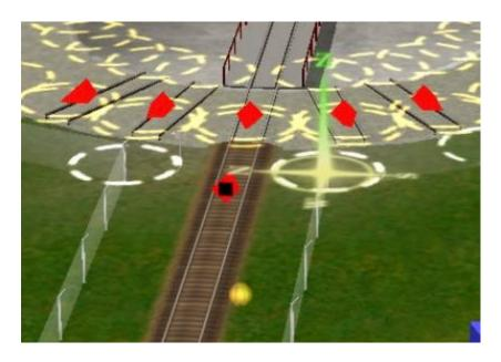
Remember we said earlier when a loco heads toward an End-of-Track marker, it will stop about two car lengths away? Remember that? The dwarf signal works the same way.
