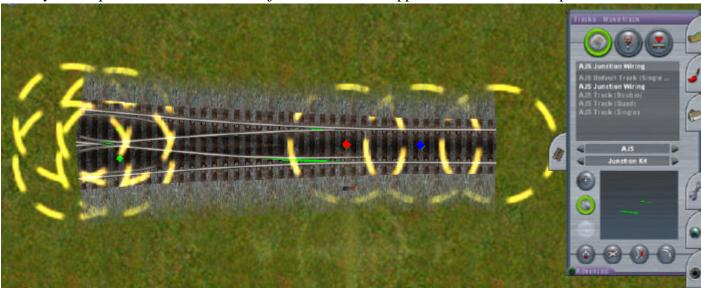
Drag the junction lever to the central diamond, align the tracks and release. Select Track / Trackside / Default Junction Direction and test the point.
