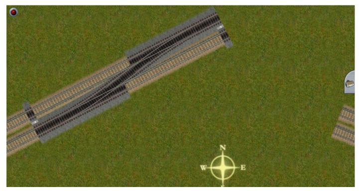
For twin track you must move the assembled template on to the track rather than vice versa. You can rotate the template together with any attached tracks until the angles are a close enough match to enable the snapping mechanism to work.
